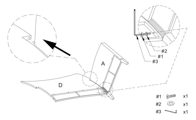
Step 2. Attach seat panel (part C) to right arm panel (part A) and back panel (part D) using bolts (part #1), flat washers (part #2) and allen wrench (part #3).
