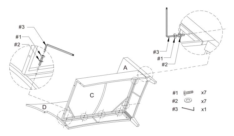
Step 3. Attach left arm panel (part B) to back panel (part D) and seat panel (part C) using bolts (part #1), flat washers (part #2) and allen wrench (part #3).
